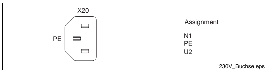
Fig. 7-21: Pin assignment of the 230/115 VAC connection X20
